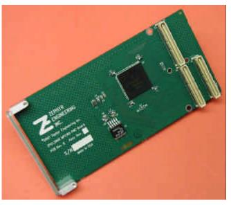
The **ZPCI.3900** MPC190 Security Processor PMC module from Zephyr Engineering, Inc is a high-performance encryption/decryption engine on a 64-bit 66 MHz PMC form-factor card.
