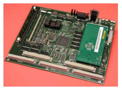
The **ZPC.1900** Security Processor Development Platform from Zephyr Engineering, Inc is a high-performance platform suitable for software development of security applications.
